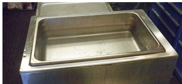
For smaller scale production and testing, a food warmer tray can be used as a dye tank.
