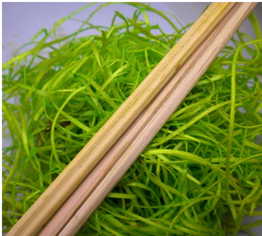
3) After one minute in the solution, the dye is quickly adsorbed onto the excelsior, while the reeds show little coloration.
